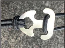
The other minor modification I made to the wing was to add a bungee clip from Andrew Goring. I find this to be a particularly nice way to keep the wing tip bungees connected together.
